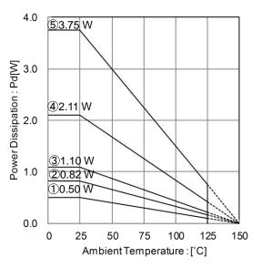
Figure 15. Thermal Reduction Characteristics
