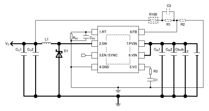
Exposed die pad is needed to be connected to GND.
