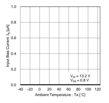
Figure 7. Input Bias Current vs Ambient Temperature
