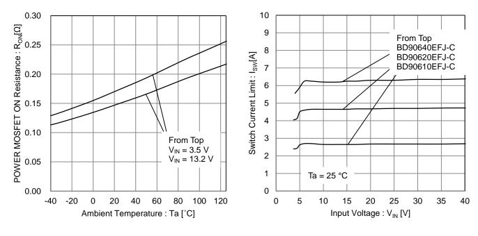
Figure 3. POWER MOSFET ON Resistance vs Ambient Temperature
