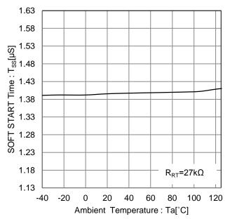
Figure 8. SS Time vs Ambient Temperature
