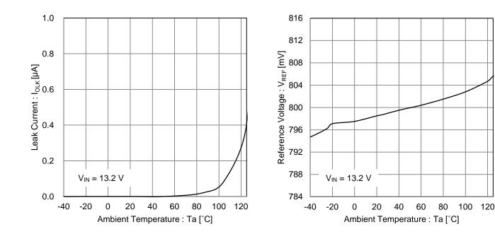
Figure 5. Leak Current vs Ambient Temperature
