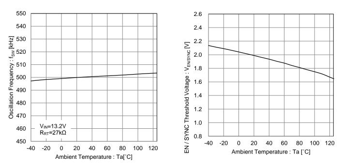
Figure 9. Oscillation Frequency vs Ambient Temperature
